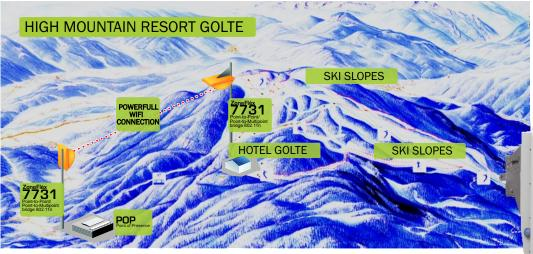
With implementation of a single pair of Ruckus Wireless ZoneFlex 7731 Wi-Fi bridga, High mountain resort Golte got connected to a POP (Point of Presence). The connection runs alongside the cable car route, total distance is 4 km with 1000 meters of altitude change.
